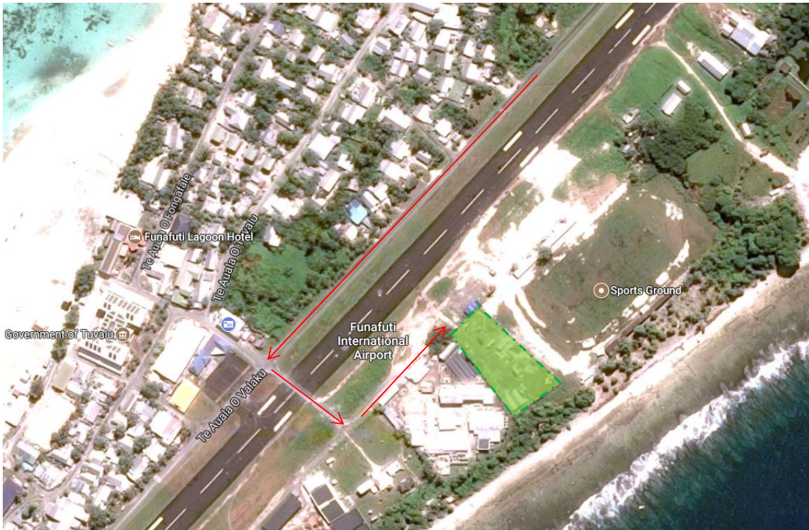
Figure 2: Path to Site Area: This figure shows the common path for deliveries to and from site from the Site Area. All bulk materials are to be stored on the site.
